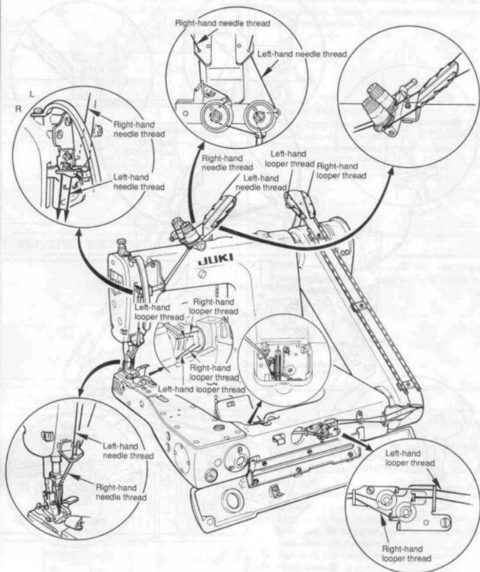
Thread the machine head in the order shown in the figure.
